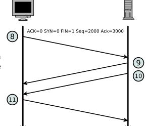
3. The diagram shows the termination of a TCP connection. Complete the table.
