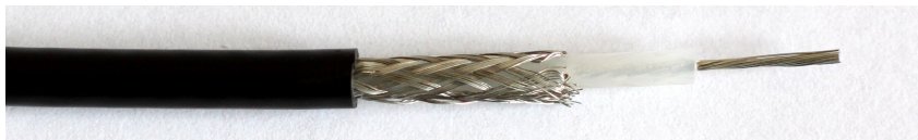
↑ Pastic jacket (PVC) ↑ Outer conductor 'Shield' (aluminium) ↑ Insulator (PE) ↑ Inner conductor 'Core' (copper)
