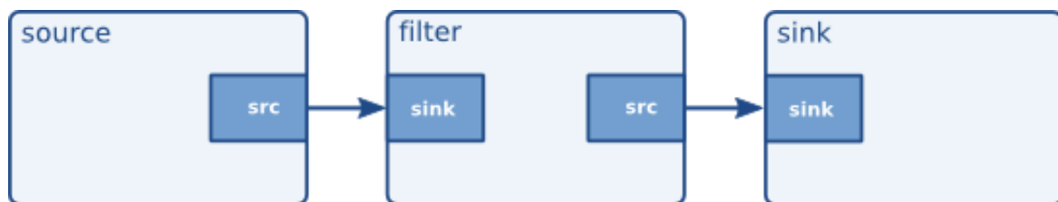
Abbildung 6: GStreamer, Elemente, Pads, Pipeline [26]
