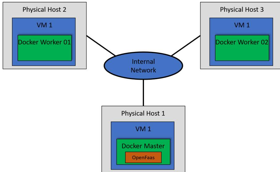
Figure 3: Multiple host setup for the test cluster
