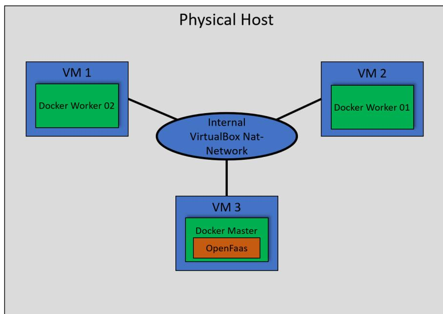
Figure 2: One host Setup for the test cluster
