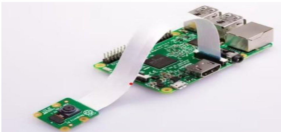
Figure 4: Connect the Raspberry Pi Camera Module v2
