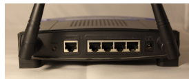
The two pictures below show a Linksys WRT54GL Wireless-G Wireless Router with a WAN port and a 4-port switch
