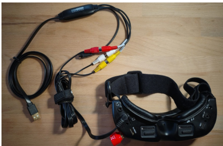
FPV goggles connected to a video grabber for processing the live video stream on a computer
