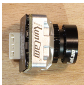
Figure 1.12: RunCam Phoenix 2 Analog Camera 1000 TVL 19x19 mm (Top and Back)
