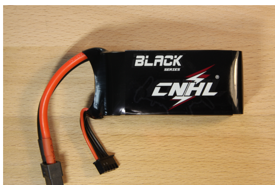
Figure 1.6: 4S Lithium-Polymer Battery with 1500mAh Capacity and 100 C Capacity Rate
