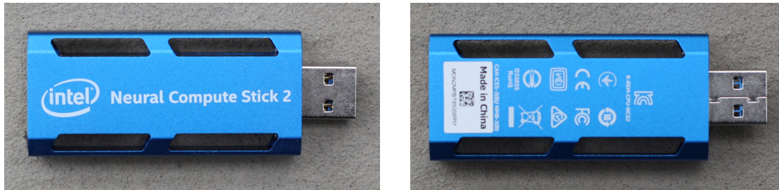
Figure 4.3: Intel Neuronal Compute Stick 2 (Front and Back)
