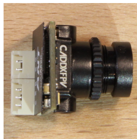
Figure 1.11: Caddx ANT Nano Analog Camera 1200 TVL 14x14 mm (Top and Back)
