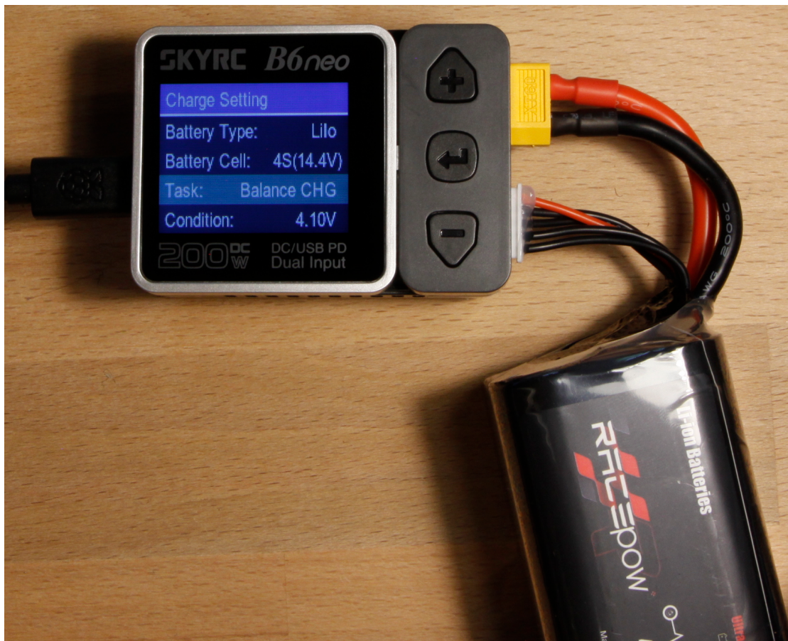
Figure 3.1: Balanced Loading of a Li-Ion Battery
