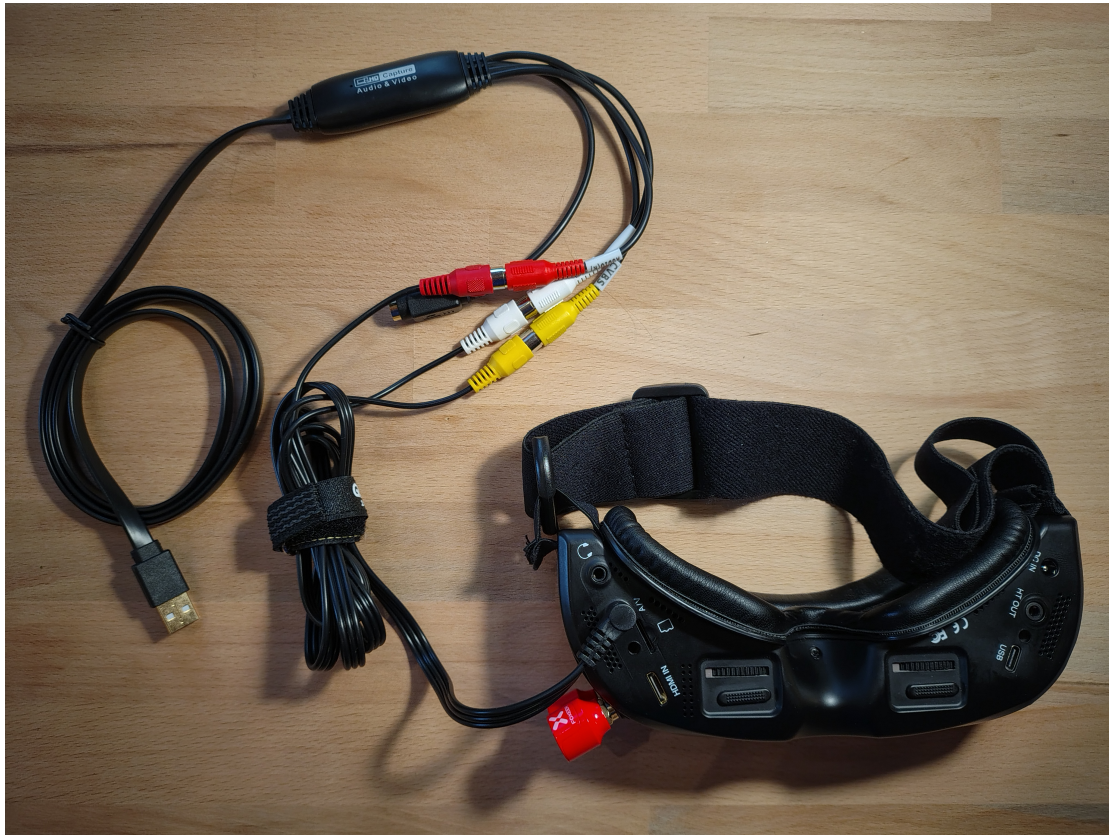
Figure 4.5: Video Grabber Device connected to the A/V Port of an FPV Goggle
