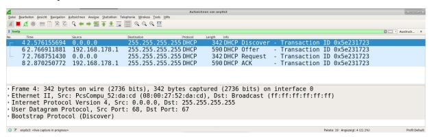
a) Sketch inside the Message Sequence Chart (MSC) the sequence of the IPv4 address assignment by using DHCP. Specify for each transmitted message the transmission direction, IP addresses of sender and receiver, as well as DHCP message name.
