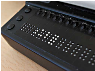
Figure: A braille terminal for blind persons
