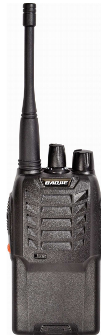
Picture of a handheld transceiver „walkie-talkie“
