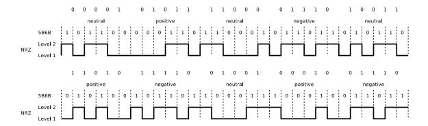
4. These signal curves are encoded with NRZI and 4B5B. Decode the data.
